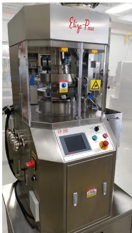
Photo 2: The EP-200 D-size tablet press uses 8 stations with D tooling to produce up to 14,400 tablets per hour.
