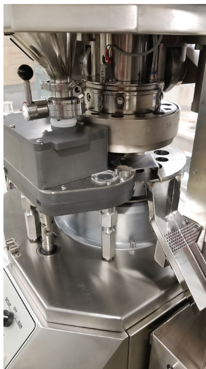
Photo 3: The B/D combination turret shown accepts B and D tooling, providing manufacturing flexibility.
