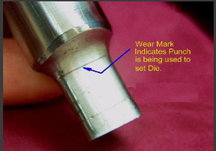
Punch is being used to set dies in press.
